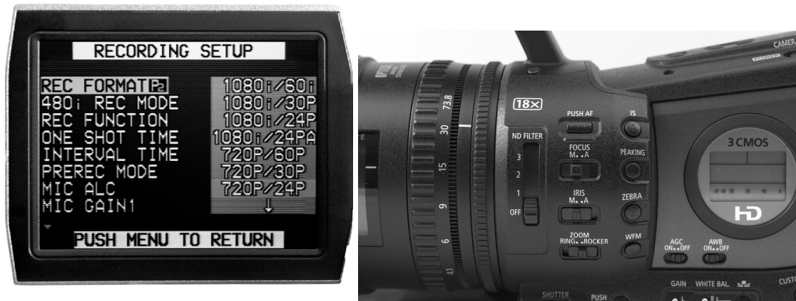
Figure 8-23 Some video camera functions are embedded inside menus accessible on the LCD screen (left), while other more commonly used features (like the manual overrides for focus and iris) are sometimes found on the camera's body (right).
