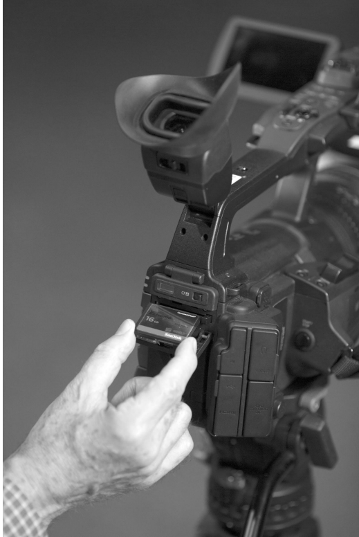
Figure 8-21 File-based recording on solid-state memory cards, like the SD card pictured above, offers many advantages over tape and is now the standard. The camera pictured, the Canon XF300, has 2 slots to allow for longer, continuous recording.
