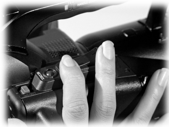
Figure 8-20 The servo zoom rocker-switch allows the camera operator to glide through the entire range of focal lengths available on the lens. High-end cameras provide speed adjustments for this switch, allowing even greater control.
