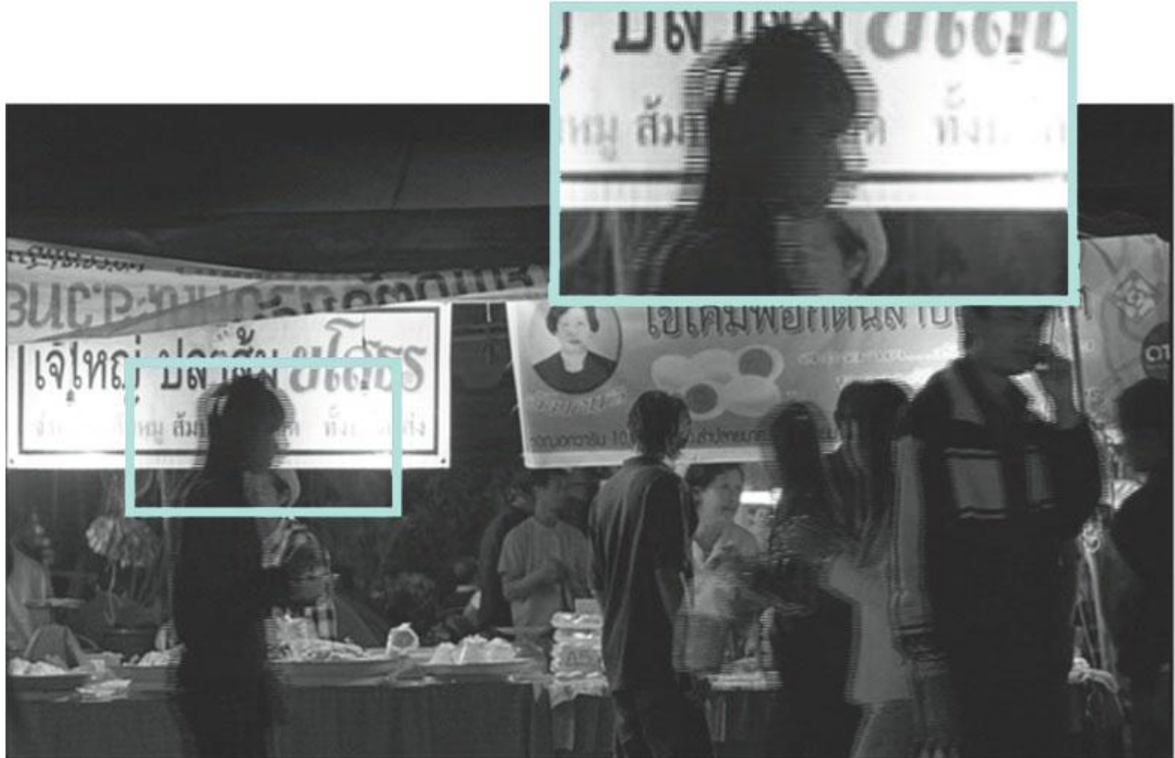
Figure 8-9 When interlaced video is shown on progressing displays, a “combing” artifact occurs at the edges of moving objects caused by the displaced scan lines (notice that the stationary objects do not show any combing).
