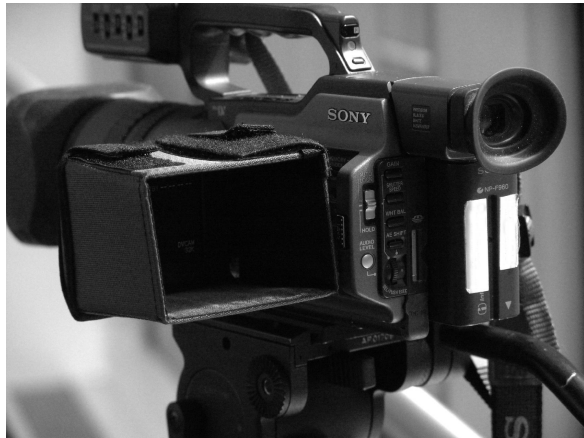
Figure 8-18 An LCD monitor hood keeps sunlight from washing out the LCD screen when shooting in sunny locations.
