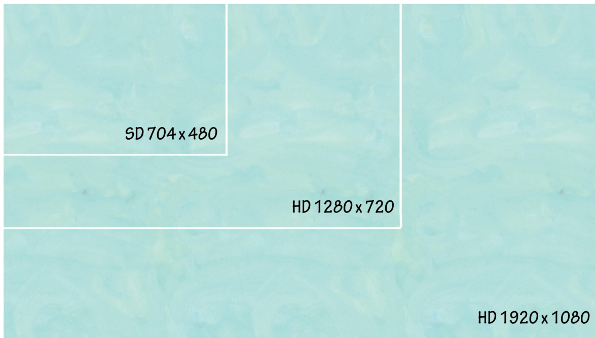
Figure 8-6 The resolution of video formats can be roughly determined by multiplying the horizontal by the vertical pixels. This illustration shows the relative resolution capabilities based on pixel count.
