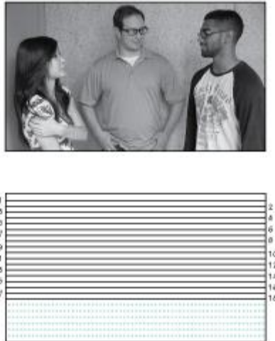
Figure 8-8 Progressive scanning draws a full frame of video, from top to bottom, without skipping any lines.
