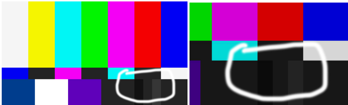
Figure 8-38 In this typical color bar display, the brightness of the three small bars on the lower right (called the pluge, from picture line-up generation equipment) can be used to set brightness level. In the closeup section of the bar display (right), the setting has been adjusted so that the difference between the two bars on the left of pluge almost disappears. See color insert.
